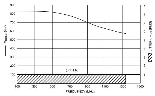
Figure 2. F<sub>max</sub>/Jitter
